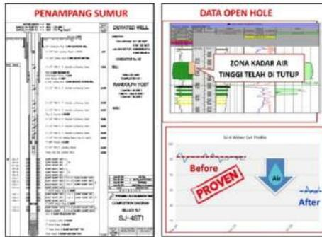
Gambar. Metode penutupan sumur setelah inovasi Program COPS (Co Log & Production Logging Tools Survey)
