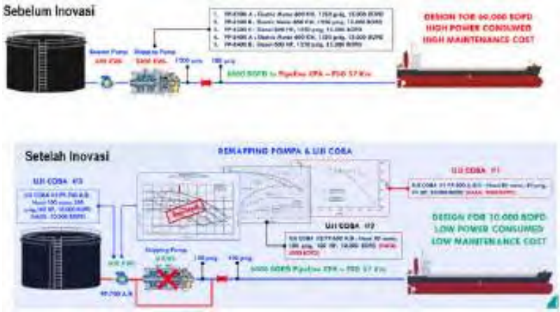
Gambar. Skema inovasi Program REMPOST (Remapping Pompa Operational)
