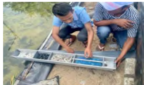
Gambar. Roughing Filter (HRF)
