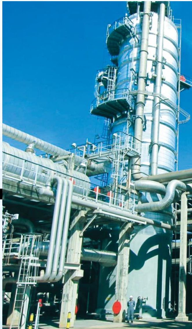
Amine Reboiler dan Amine Regenerator di Acid Gas Removal Unit (AGRU)
